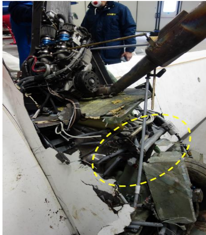
Photo 12: airbrakes torque tube damages.
