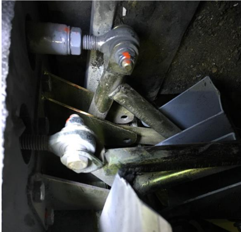
Photo 14: left wing airbrakes crankshaft , rotational axis missing.
