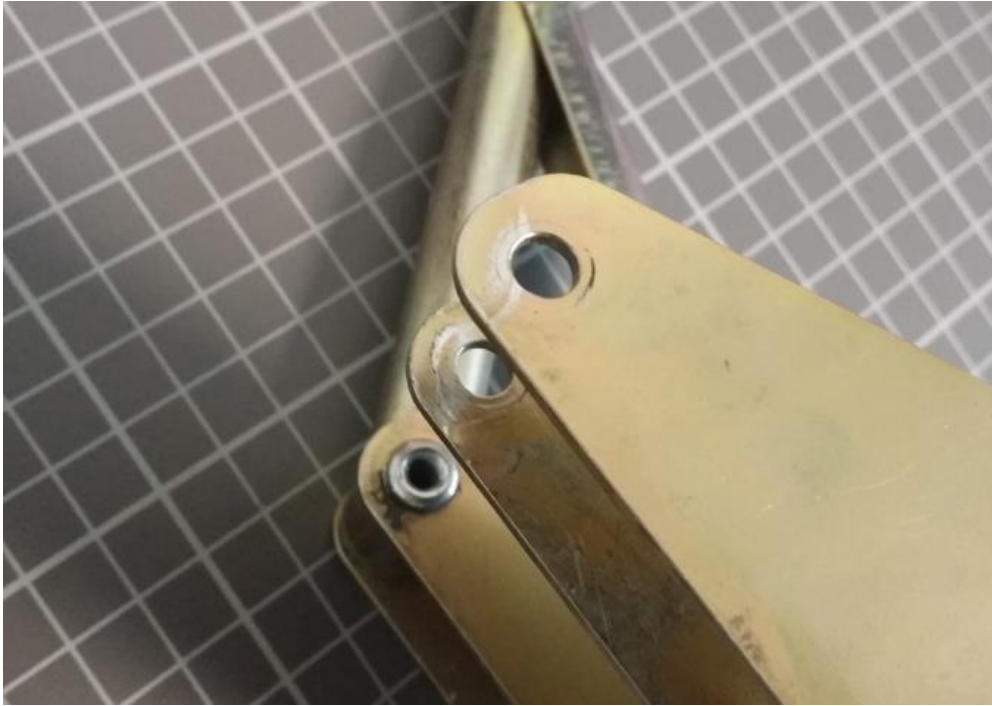
Photo 18: traces of rotational axis on left wing crankshaft supports.
