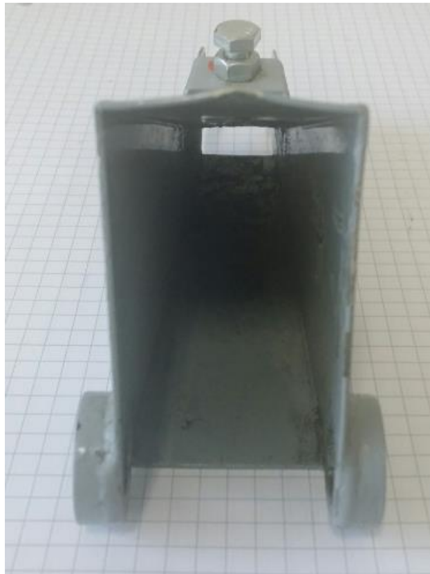
Foto 16: left wing crankshaft funnel damaged.
