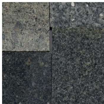
Examples of Purbeck stones: clockwise from left: some Purbeck marbles; Thornback; Grub, Freestone; Downsvein. The limestones vary in hardness, colour and fossil content according to their bed.
