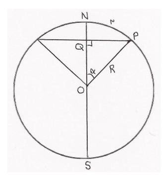
R is radius of Earth (measured from the centre of the Earth at O) Arc NP (r) is effective radius of the estate α is the polar angle of the estate perimeter
